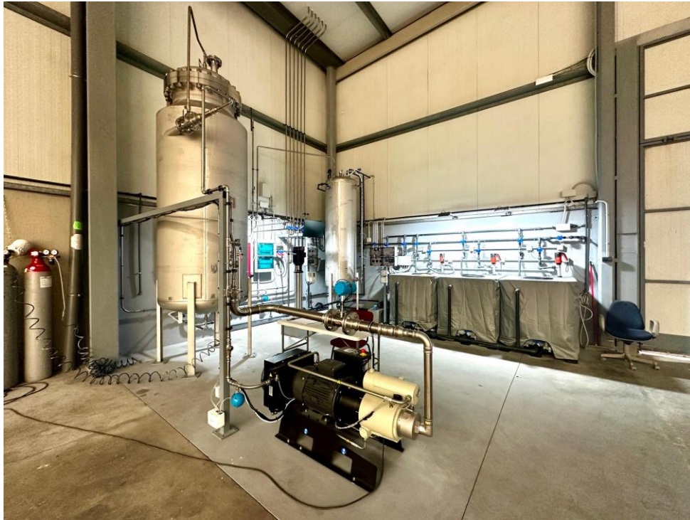
Pilot single-stage biogas purification system with CO 2 utilisation and product recovery in Spain (2025)
